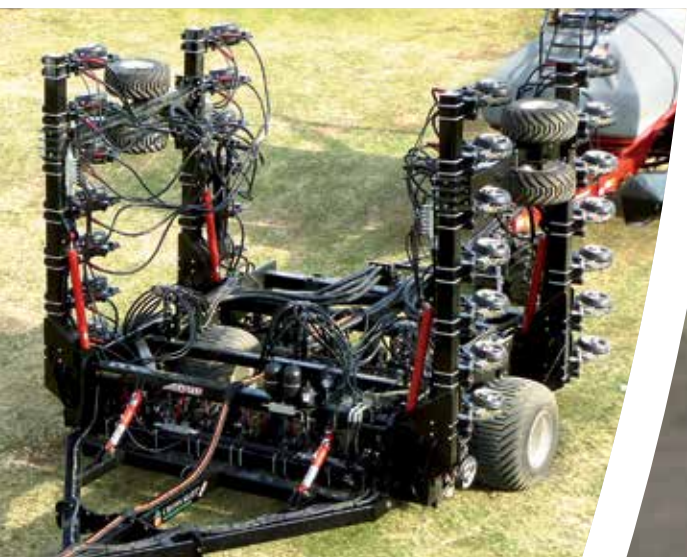
14m Cross Slot folding toolbar
