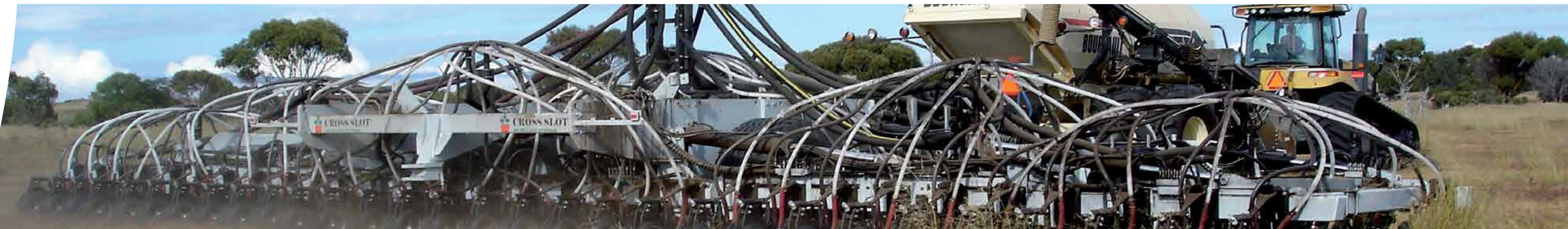
18m Cross Slot bi-folding (5-plex) toolbar
