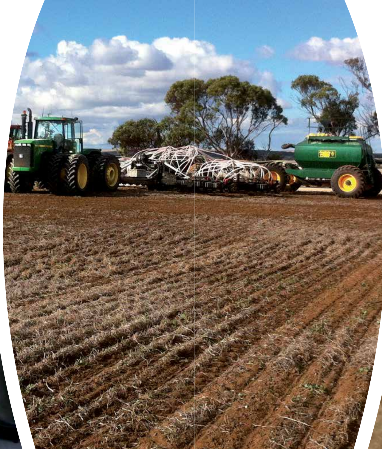
12m Cross Slot folding toolbar
